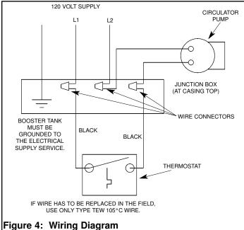
Electrical wiring must be in accordance with local codes; or in the absence of local codes with the National Electrical code ANSI/NFPA 70 or The Canadian Electrical Code, as applicable.
